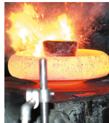
A billet is pre-formed for a ring, on a VPE 800.
