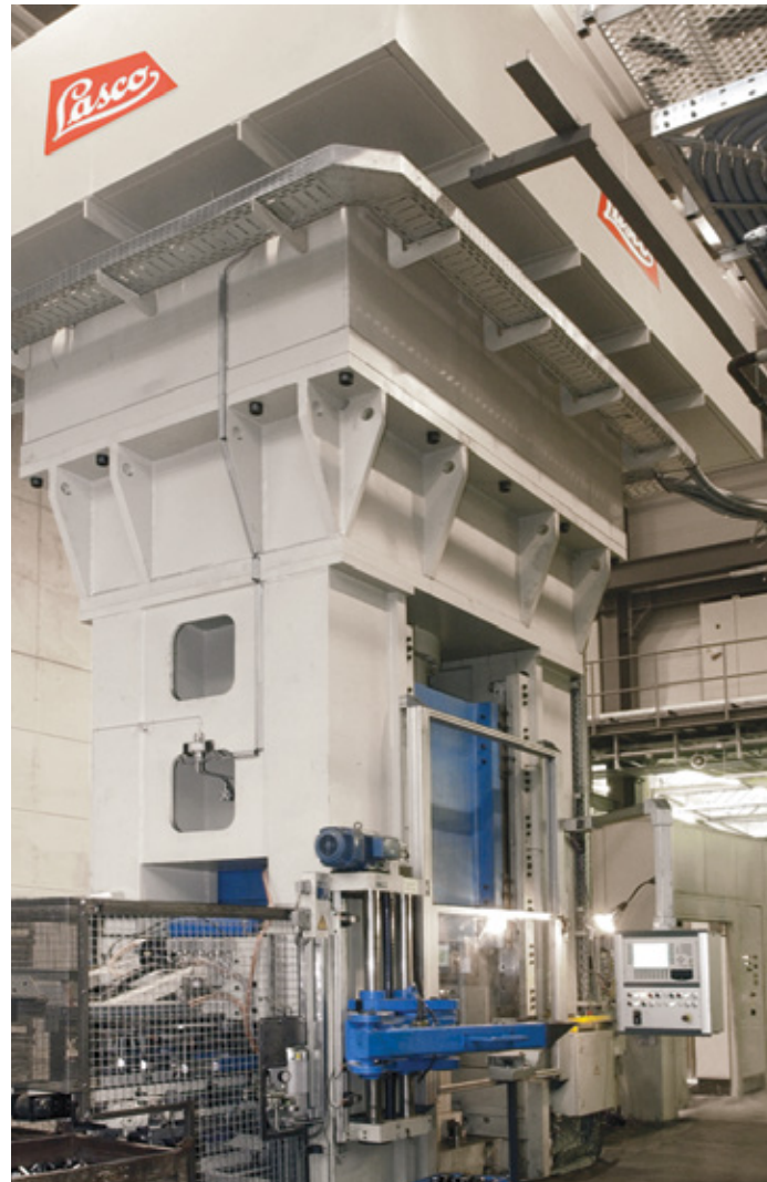
Illustrated is a LASCO KFP cold extrusion press of 1000 tonnes capacity for extrusion of automotive parts.
